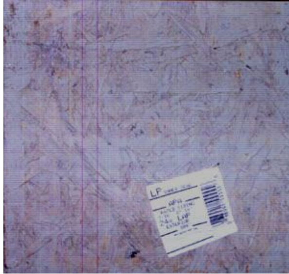
LP Siding backside pattern with large wood chips.
